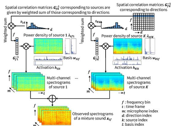
Fig. 1. The generative story of multichannel NMF.
