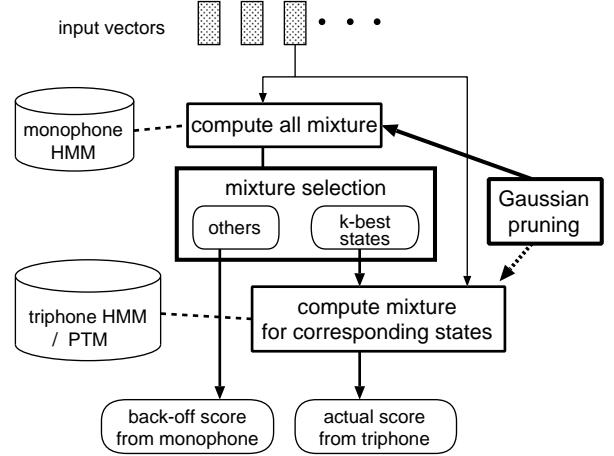
**Fig. 1.** Mixture Selection using Context-Independent HMM
