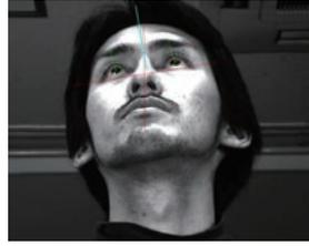
Gaze tracking result (This image was captured by the camera located under the screen.)
