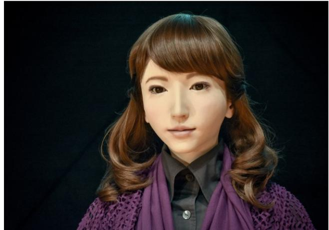
Figure 1. Photograph of ERICA, the android platform presented in this work.
