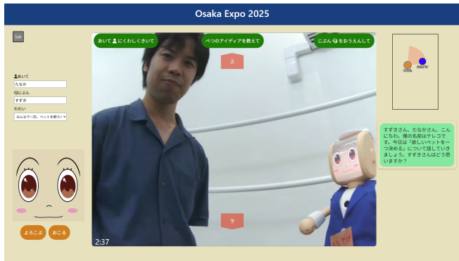
Fig. 4. Screenshot of operator's GUI, with the user on the left and T-AUTO on the right. Green buttons at the top of the GUI are for sending commands to T-AUTO . The scenario is designed so that both participants are displayed within the camera frame.
