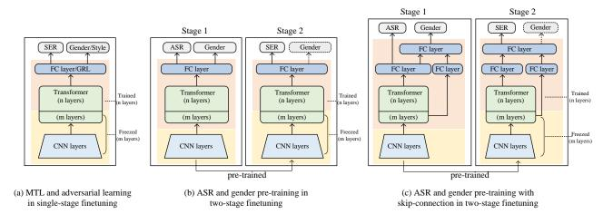
Figure 1: Network structure of wav2vec 2.0-based models. In two-stage finetuning methods, we finetune all the Transformer layers in stage 1 and n Transformer layers (pink part) in stage 2.
